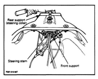
Position steering stem arm and support onto steering stem.
